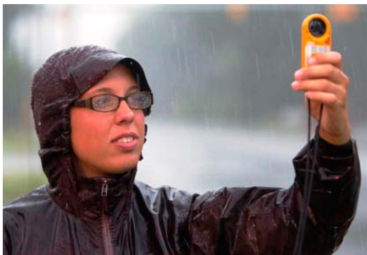
Graduate student Kelsey Mulder using a Kestral handheld instrument which measures wind speed and surface pressure. Cliff Hollis, ECU News Services.
