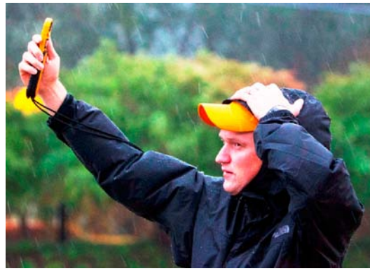
Undergraduate student Noah Poe using a Kestral handheld instrument which measures wind speed and surface pressure. Cliff Hollis, ECU News Services.
