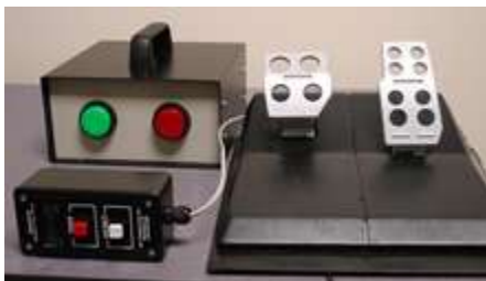
RT-2S is the new brake reaction device tested.
