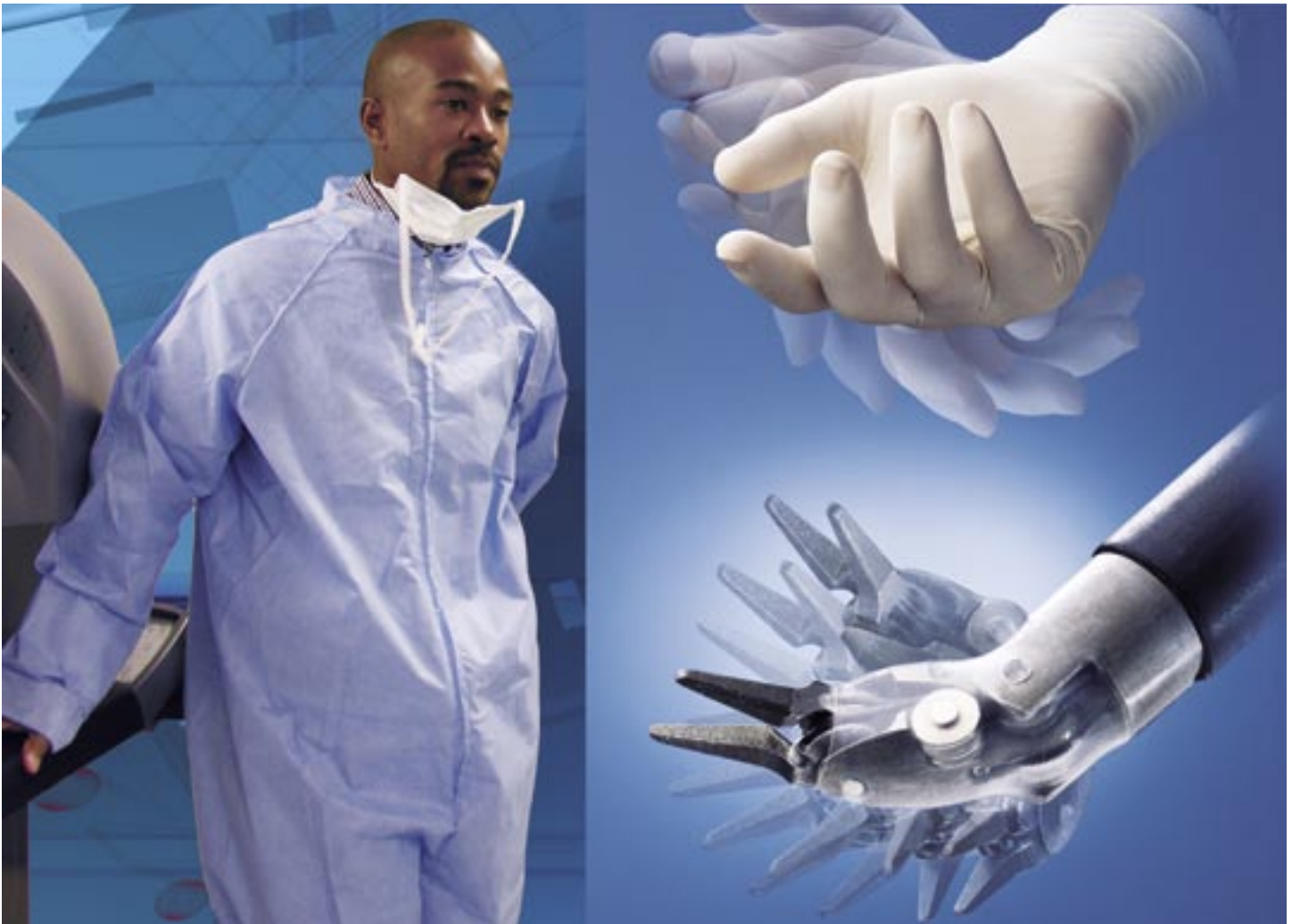
Dr. Dieter Bruno with an illustration of the robotic wrist used in robotic surgery. Traditional laparoscopic instruments are straight and do not bend. EndoWrist instruments move like a human wrist, allowing increased dexterity, maneuverability and precision.
